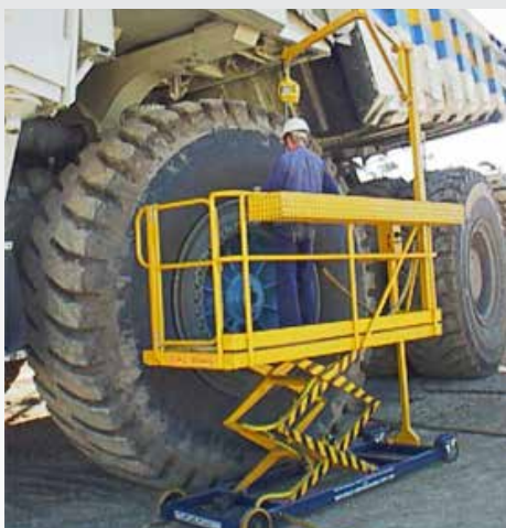
Trilift® Variable Height Work Platform in use
