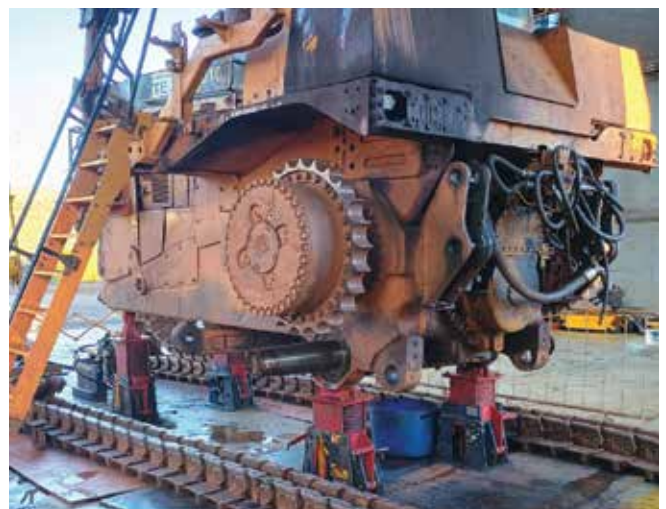
Two sets of Trilift® Jack Stand Model 100 supporting a CAT D10T
