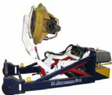
Differential removal using the Trilift® Differential Removal Jig and the Trilift® Transmission Hoist
