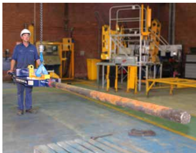
Trilift® Component Balance Tool and Axle Adaptor in use with overhead crane to remove a haul truck axle
