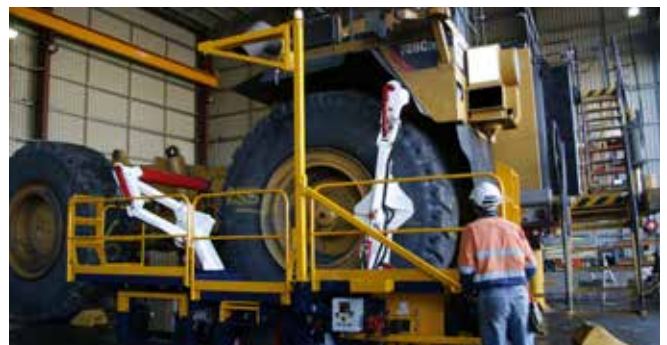
Trilift® TH15000 Workshop Tyre Handler removing Cat 789C tyre
