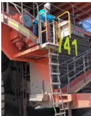
Model EE Ladder shown fitted to excavator in the down position
