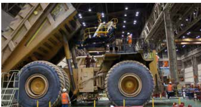
Trilift® Cat 797 Transmission Hoist removing transmission
