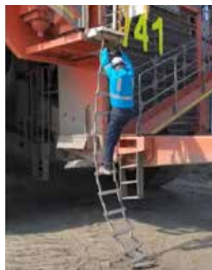
Model EE Ladder shown fitted to excavator in the down position
