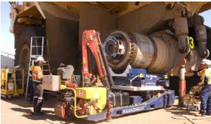
Terex MT6300 Wheel Motor removal using the VWT XC30 with a Universal Large Wheel Motor Jig
