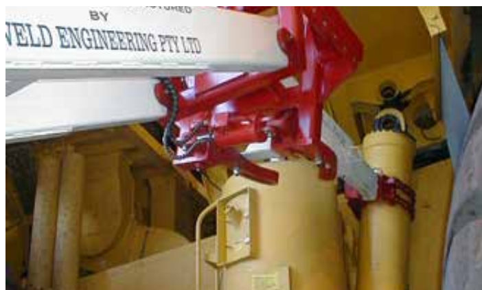
Hoist cylinder removal with VWT 15 and Multijig 15 with Universal Cylinder Clamp
