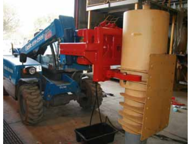
Trilift® Universal Quick Hitch on a Genie removing a strut
