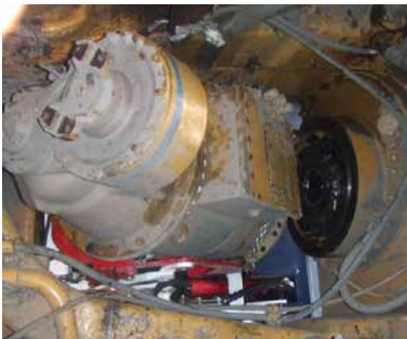
The Trilift® Transmission Hoist MKII lowering the transmission through the bottom of the chassis.
