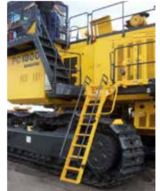
Safe-Away® Swing ladder in the down position on a PC1800.
