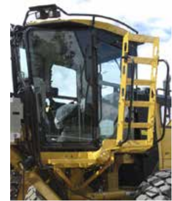
RotorStep GM Ladder shown fitted to a 16M Grader
