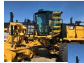
RotorStep M3 Ladder shown fitted to a Cat 18M3 Grader
