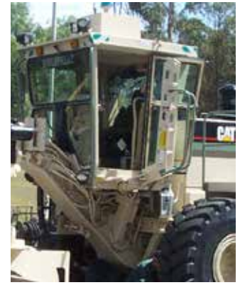
RotorStep G Ladder shown fitted to a Cat 16G Grader
