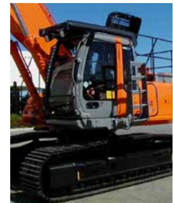
RotorStep L Ladder shown fitted to a Hitachi EX350 excavator
