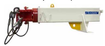
The **Universal Cylinder Clamp** (*Part No. TL02006*) when used in conjunction with the Multijig 15, is designed to assist with the safe and efficient handling of large hydraulic cylinders, including hoist cylinders and rear struts.
