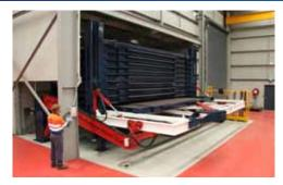
Hedweld has designed and manufactured a 150T Material Handling Station consisting of 11 cassettes, which accept material dimensions of 2400x6000mm, with thicknesses ranging from 6mm up to 50mm. This product offers:
