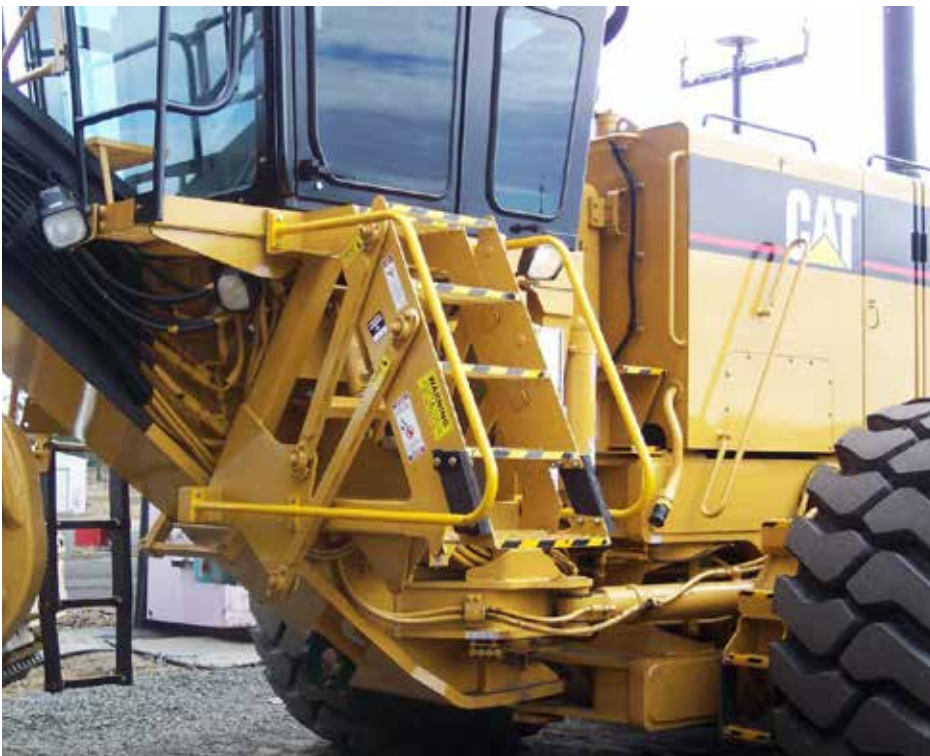
EL-24H Electric Ladder shown above in the retracted position. This picture shows you the specialised mounting brackets.
