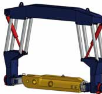
Dozer Track Frame rotation for safer maintenance
