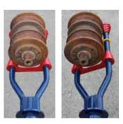
The Component Balance Tool also includes an Axle Adapter (Part No. HW75366) to assist in the removal of axle.
