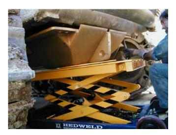
The top plate of the Belly Pan Hoist has been pre-drilled to accept a range of component specific Trilift® jigs and other tooling, making this tool quite versatile in the removal of small OEM vehicle components. These include:
