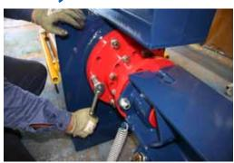
It only takes a few minutes to attach and detach the Counterweight (Part No. HW75327) from the Balance Jig.
