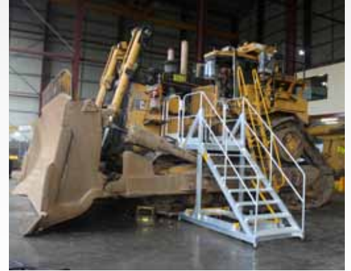
Dozer Access Platform
