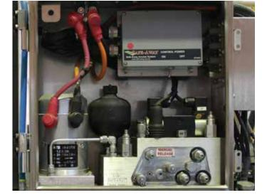
The **Safe-Away® 2009 Series Power Pack** is driven by the Access Control System. The hydraulic Power Pack is neatly mounted vertically on the side of the Access System. It includes:
