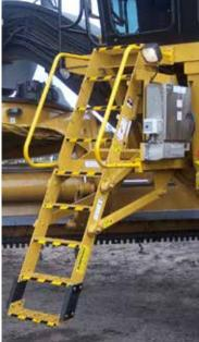
Cat 24H Ladder shown above in the retracted position. This picture shows you the specialised mounting brackets.
