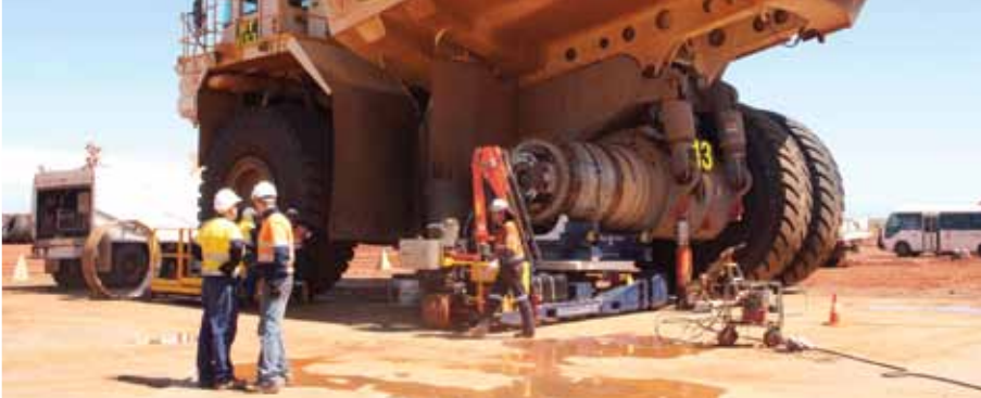
Trilift® Variable Work Table and Universal Large Wheel Motor Jig removing a Terex MT6300 wheel motor
