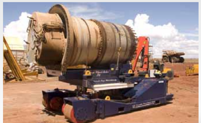
The Trilift® VWT XC30 with wheel motor removed from Terex MT6300
