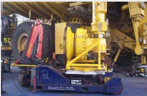
Hub & Strut removal with the Trilift® Hub & Strut jig
