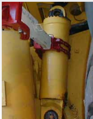
The Trilift® Universal Cylinder Clamp removing a cylinder
