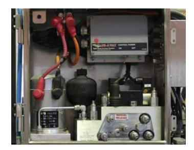
The **Safe-Away® 2009 Series Power Pack** is driven by the Access Control System. The hydraulic Power Pack may be mounted vertically, at a convenient location of your choosing, on the vehicle.
