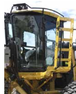
RotorStep GM Ladder shown fitted to a 16M Grader
