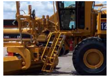
RotorStep G Ladder shown fitted to a Cat 16G Grader
