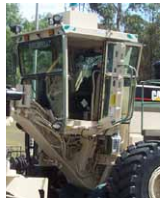
RotorStep G Ladder shown fitted to a Cat 16G Grader
