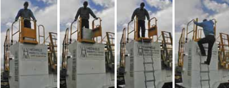
Step 1 Release lock by lifting the gate Step 2 Open gate Step 3 Push ladder out Step 4 Descend
