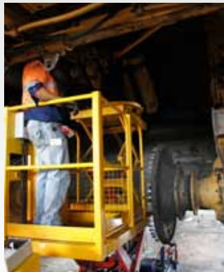
Positioning accumulator jig
