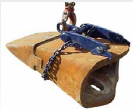
Chain N Lift fitted to a bucket tooth
