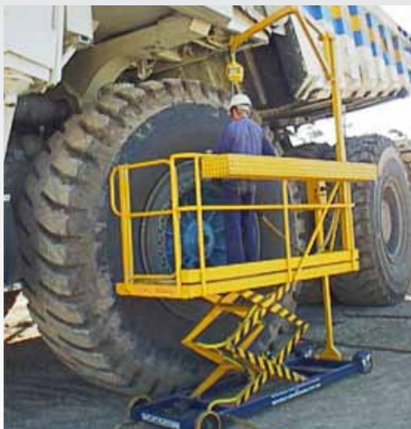
Trilift® Variable Height Work Platform in use
