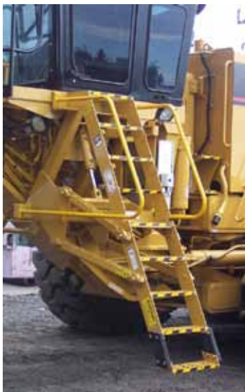
EL-24H Electric Ladder shown above in the retracted position. This picture shows you the specialised mounting brackets.
