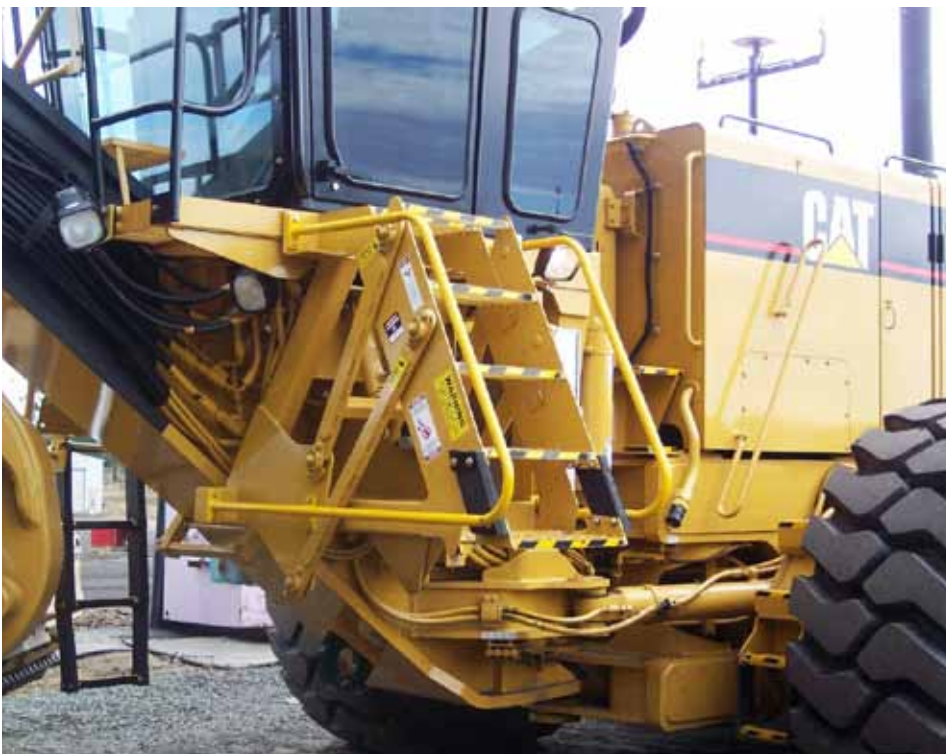
Cat 24H Ladder shown above in the retracted position. This picture shows you the specialised mounting brackets.
