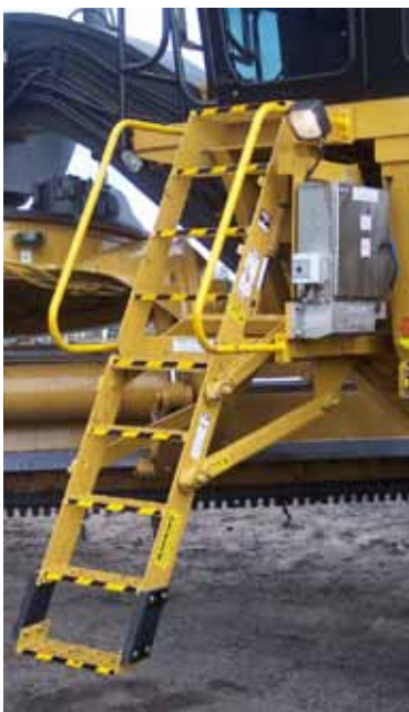
The image left shows the Cat 24H Ladder in the extended position. From this side you can clearly see the silver cabinet containing the vertical Safe-Away® 2009 Series Power Pack and the optional Boarding Light.
